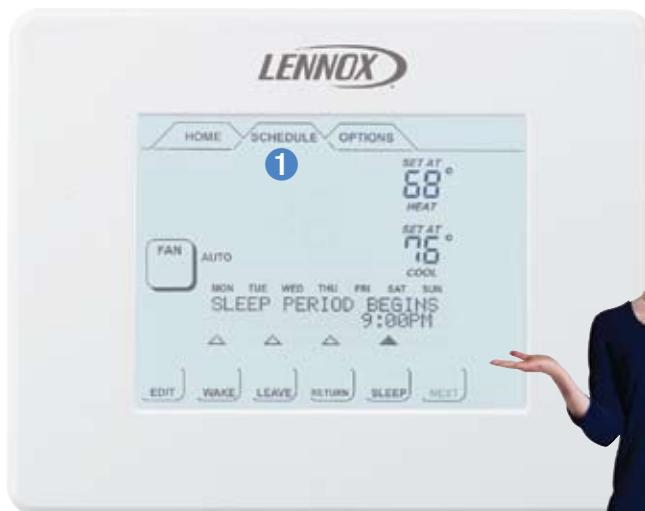
**1** **Programming mode** – Simply press the *SCHEDULE* tab to begin programming; the *EDIT* button, *NEXT* button and *ARROWS* are used to select and enter your desired settings
